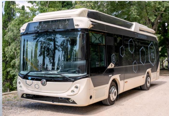
Designing and creating, entirely in Italy, Hydron is a unique hydrogen bus, the result of ten years of research. It is an innovative vehicle, the only one in Europe capable of transporting up to 48 people, in just eight metres, with an autonomy of up to 400 km that integrates the benefits of electricity with the sustainability of hydrogen, all in a single bus.
