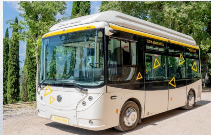
SIXTRON is a true Full Electric urban bus measuring 6 meters in length. Small on the outside and spacious inside, it's perfect for urban environments, with a low-floor platform and space for disabled passengers, accommodating up to 31 passengers. It's designed to operate with zero emissions, even in the narrowest alleyways of historic city centers.
